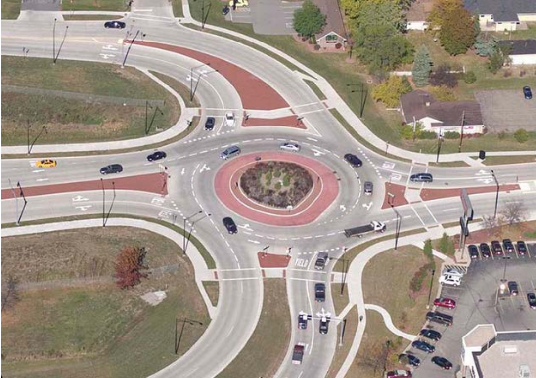
Figure 3.44 – Example of Two-Lane Roundabout with Spiral Lane to Transition Innermost Left Turn Traffic from Southern Approach Leg to Exit (Source: GHD 10 )
