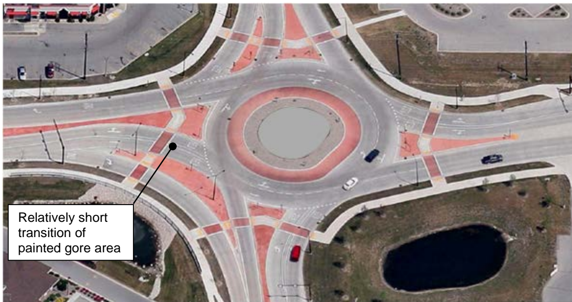
Figure 3.23 – Case 2 Roundabout (Source: RTE 11 )
