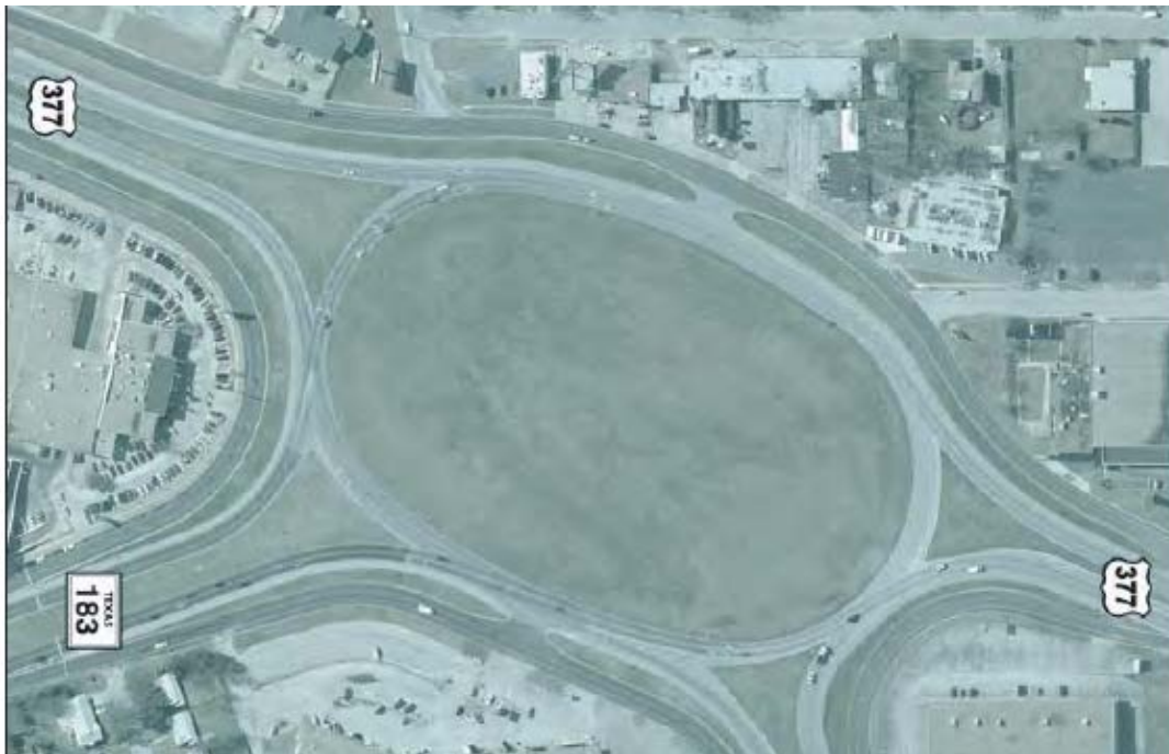
Figure 1.1 – Rotary Intersection (Source: NCHRP 672)
