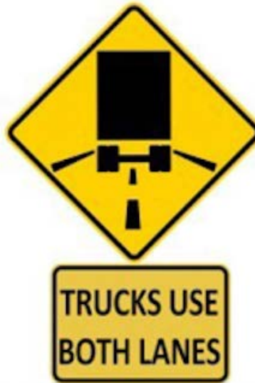
Figure 3.28 – Sample Supplemental Warning Sign to Indicate Trucks Use Both Lanes within Roundabout
